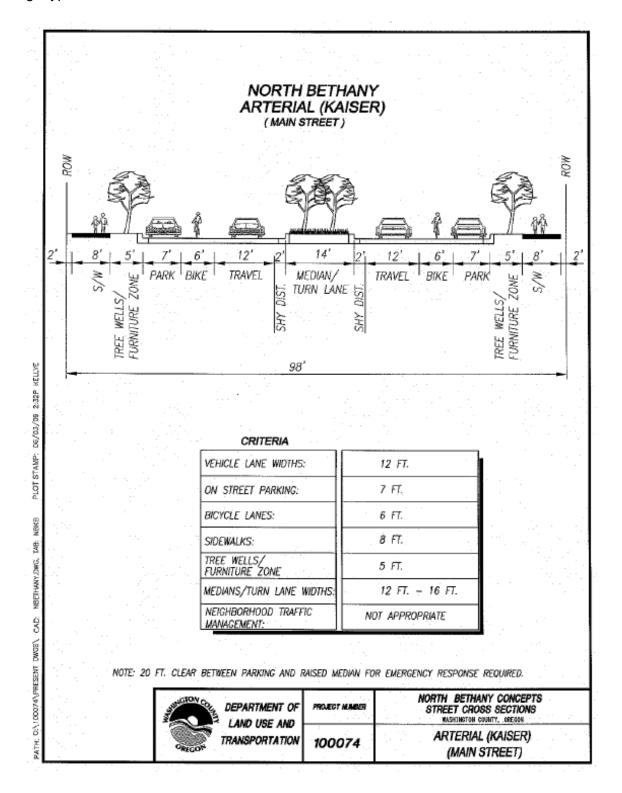
Add the following conceptual cross section detail to the North Bethany Subarea Plan for street design type AR1-c:
