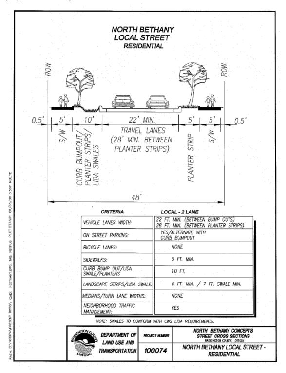
Add the following conceptual cross section detail to the North Bethany Subarea Plan for street design type PB:
