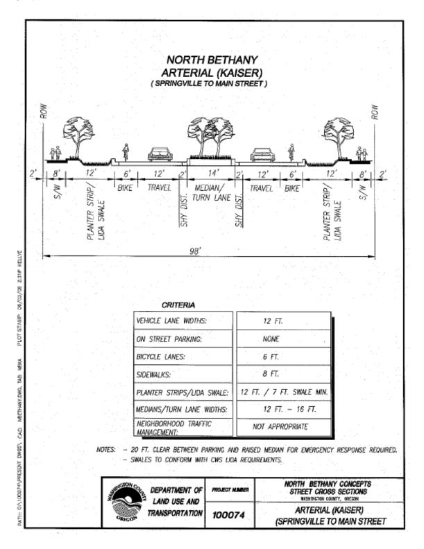
Add the following conceptual cross section detail to the North Bethany Subarea Plan for street design type AR1-b:
