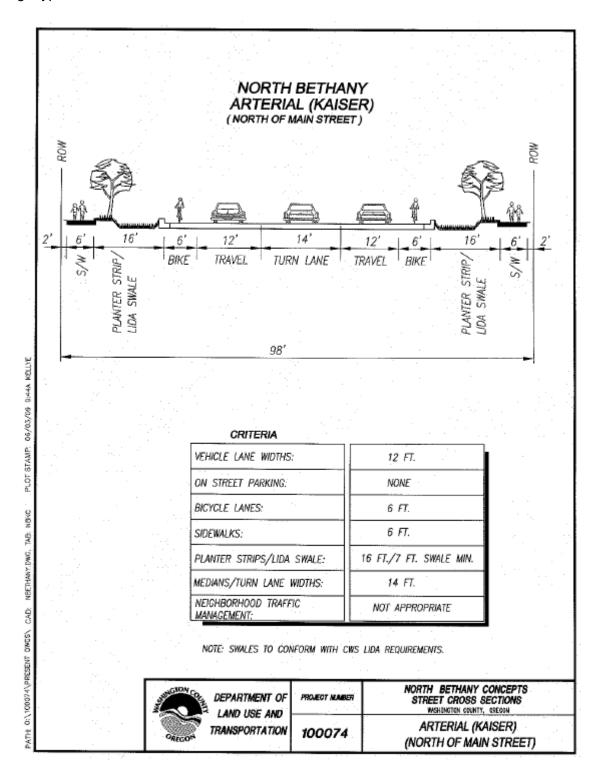
Add the following conceptual cross section detail to the North Bethany Subarea Plan for street design type AR-2:
