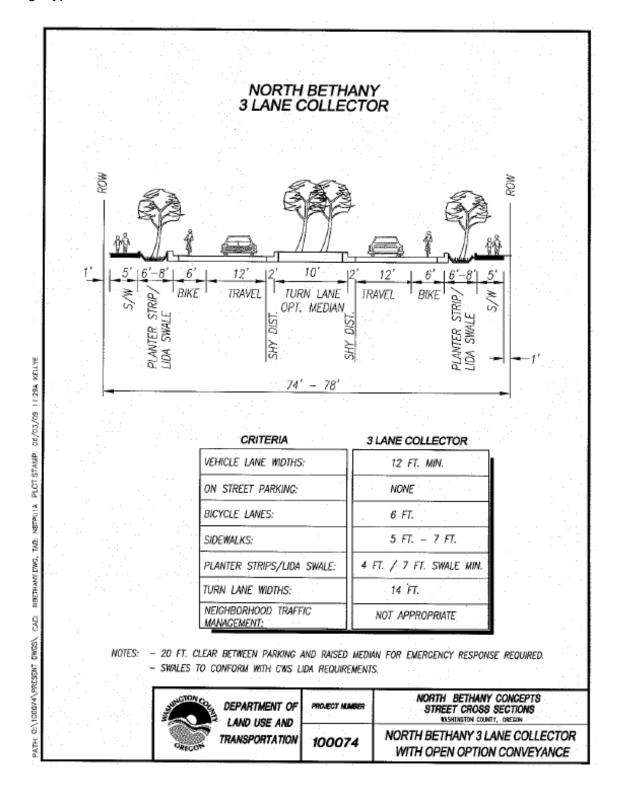
Add the following conceptual cross section detail to the North Bethany Subarea Plan for street design type CM:
